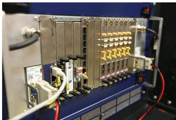
Figure 1: MTCA.4 LLRF installation at FLASH.
