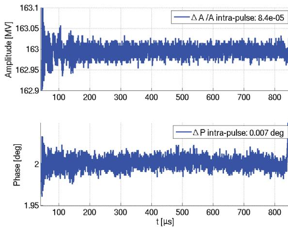
Figure 2: MTCA.4 LLRF system flattop regulation.
