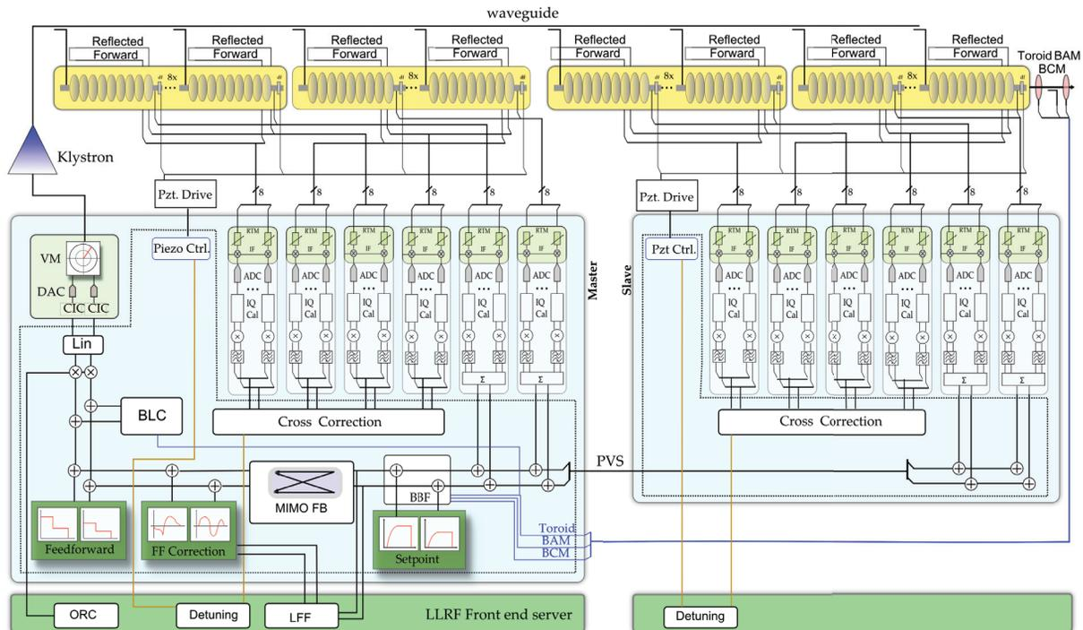
Figure 4: Functional block diagram for 32 cavity regulation.
