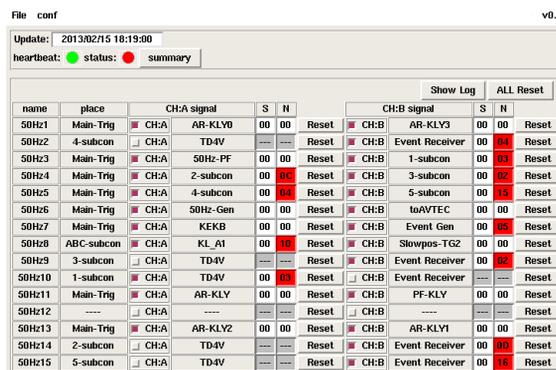
Figure 3: GUI for 50 Hz timing watchdog module.
