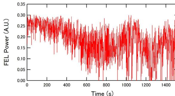
Figure 4: Time trend of the FEL output power without feedback control.
