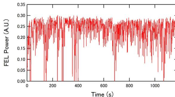
Figure 6: Time trend of the FEL output power with the BPM #2 (dX) feedback control.
