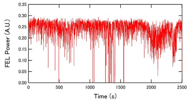
Figure 8: Time trend of the FEL output power with the BPM #2 ( $dY$ ) feedback control.
