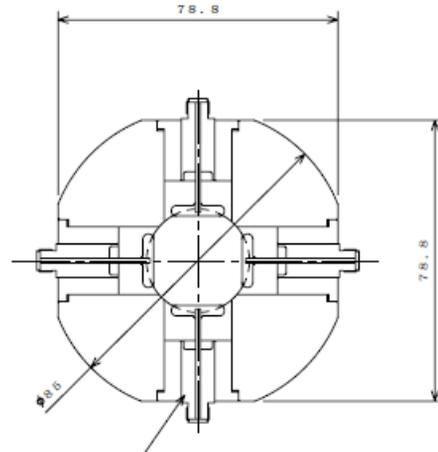
Figure 1: Cross sectional drawing of 4-button type BPM.
