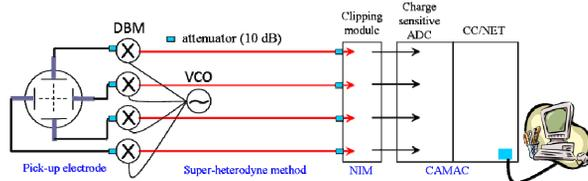
Figure 3: Signal processing diagram of BPM system.
