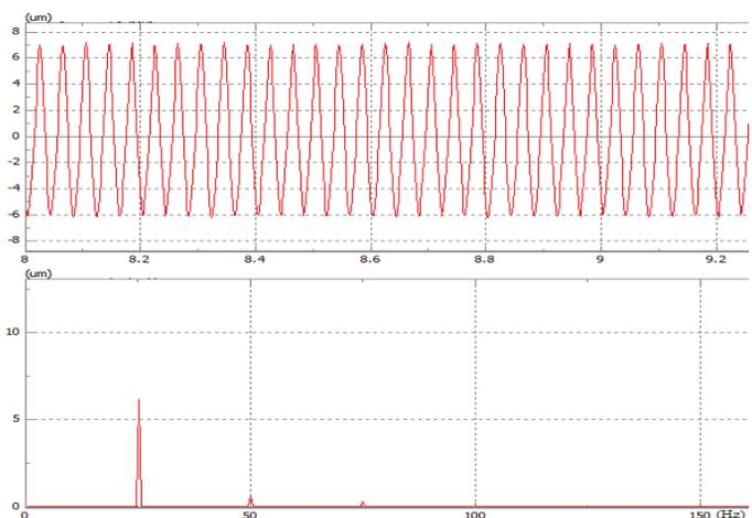
Figure 1: The dipole magnet vibration test of CSNS.
