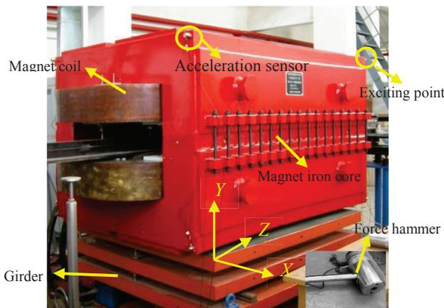
Figure 2: Experiment layout of experimental modal testing.
