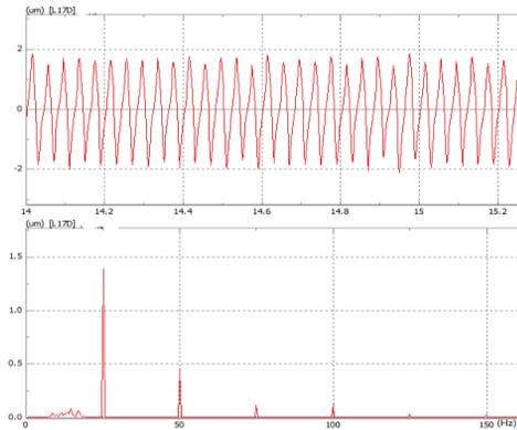
Figure 4: The vibration amplitude with isolator of dipole.
