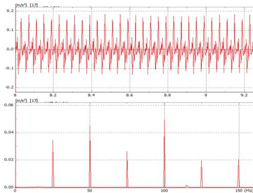
Figure 5: The acceleration amplitude with isolator of dipole vibration.
