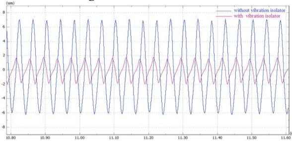
Figure 6: The vibration amplitude comparison of dipole without isolator and with isolator.
