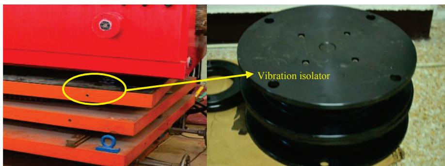
Figure 3: The vibration isolator layout of the vibration testing.
