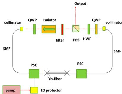
Figure 1: Schematic diagram of the 18.9-MHz all-normal-dispersion Yb-doped fiber laser, PSC: Pump signal combiner, PBS: polarizing beam splitter, SMF: single mode fiber, Yb-fiber: Yb-doped fiber, HWP: half-waveplate, QWP: quarter-waveplate.
