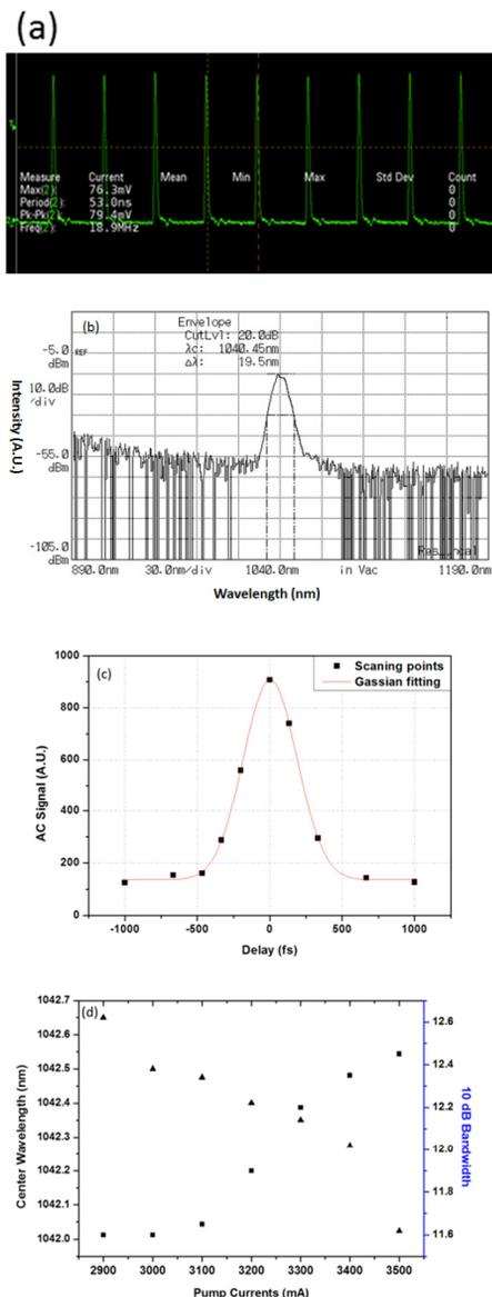
Figure 3: Output of the laser: a) oscilloscope record of the pulse train; b) typical output spectrum and the Gaussian fitting of the stable mode-locked spectrum; c) intensity autocorrelation of the output pulse; d) Stable mode-locked spectra centre wavelengths and 10-dB bandwidths corresponding to pump currents.
