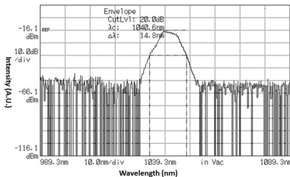
Figure 4: Output laser spectrum directly after the filter.
