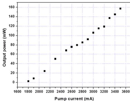
Figure 2: The output power linearly increased with the pump power.
