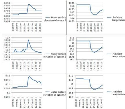
Figure 5: Temperature effects on HLS readings.
