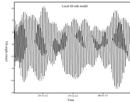
Figure 8: Modeling of local tilt tide (east-west segment).
