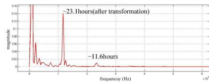
Figure 7: FFT of the difference in two sensors 22.1 m apart.
