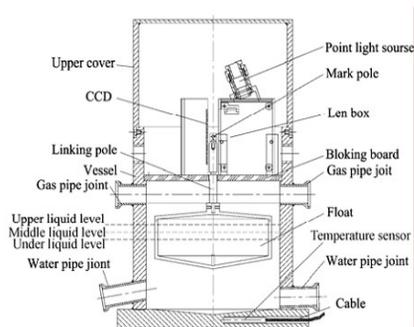
Figure 1: Structure of the sensor.
