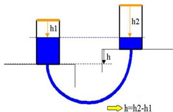
Figure 2: Measuring principle of HLS.
