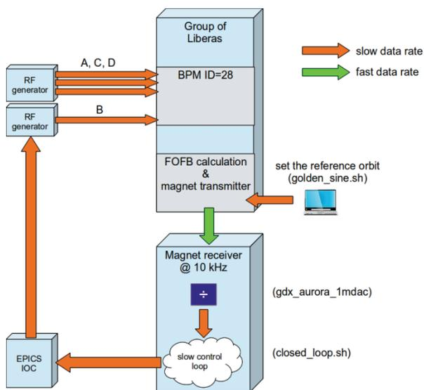
Figure 5: Experimental (slow) closed loop.
