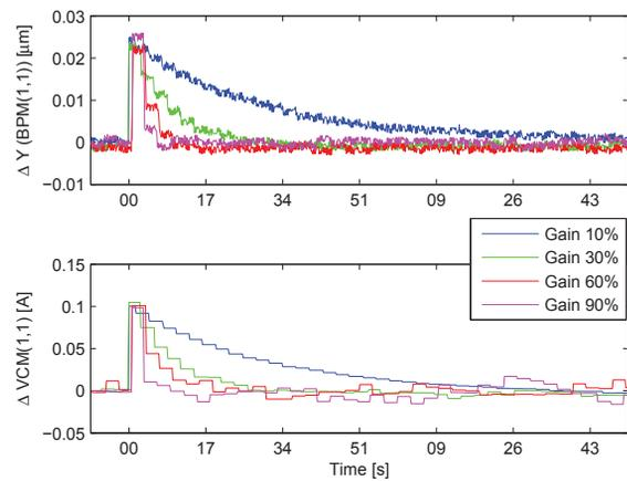
Figure 3: Response of the SOFB to a step change in the first vertical corrector. There is a small overshoot for the 90% gain.
