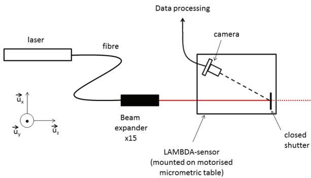
Figure 1: Top view of the experimental setup.
