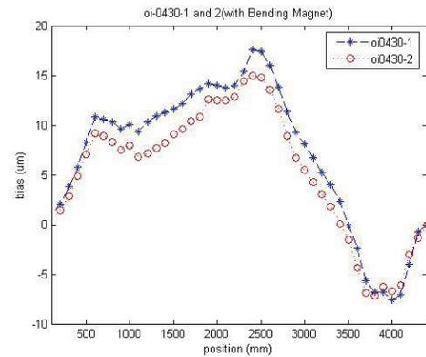
Figure 6: Typical plot of the difference in straightness of vertical direction of girders between with or without dipole magnet.
