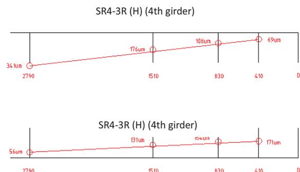
Figure 5: Typical plot of the bias of centers of magnets on 4<sup>th</sup> girder.
