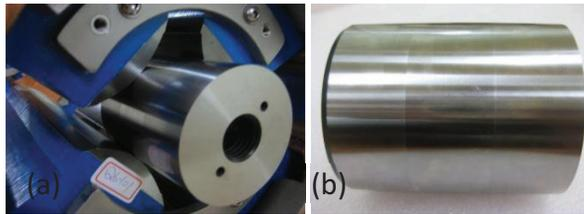
Figure 1: (a) The three-stepped arbor can be applied to insert into the quadrupole magnet. (b) The diameters of three-stepped arbor are 74.000mm, 73.991mm, and 73.973 mm, respectively.
