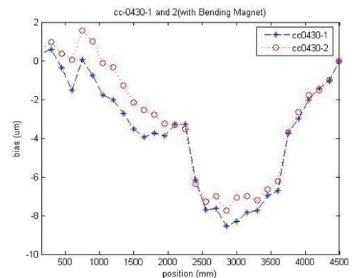
Figure 7: Typical plot of the difference in straightness of horizontal direction of girders between with or without dipole magnet.
