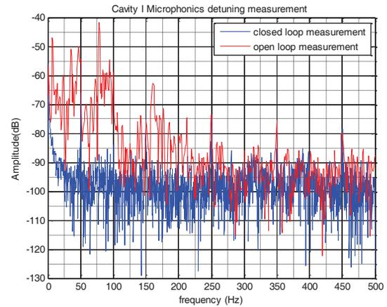
Figure 7: Cavity I microphonics test.
