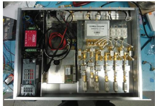
Figure 2: 19" enclosure, housing LLRF4 board and analogue components.
