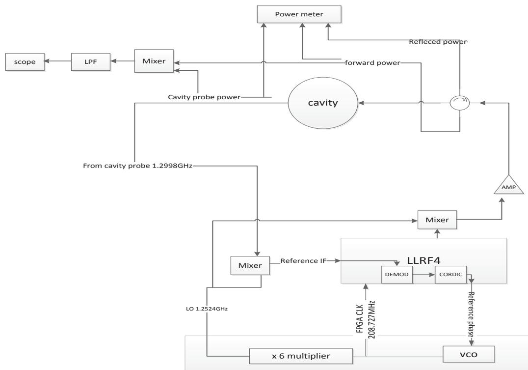
Figure 4: Digital VCO\_PLL system. LLRF4 board performs as a digital phase detector to regulate the VCO frequency.
