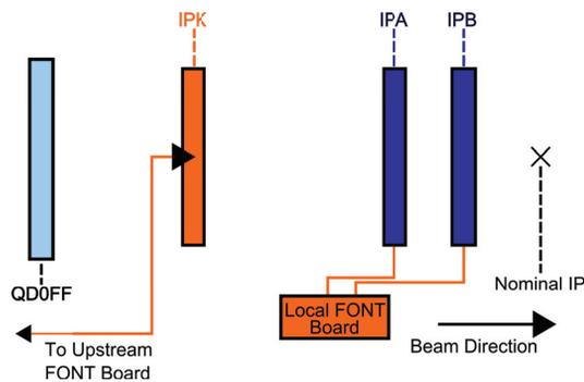
Figure 3: Schematic of IP region at the ATF2 final focus beamline showing the relative locations of the kickers, BPMs and the elements of the feedback system.
