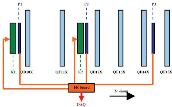
Figure 2: Schematic of FONT5 at the ATF2 extraction beamline showing the relative locations of the kickers, BPMs and the elements of the feedback system.
