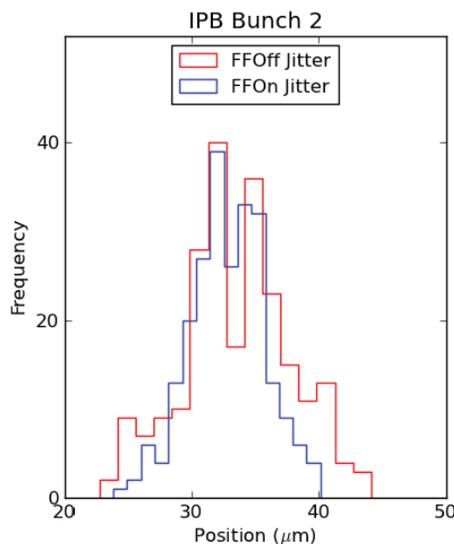
Figure 5: Distribution of vertical beam positions for the second bunch in IPB during a feedforward run.
