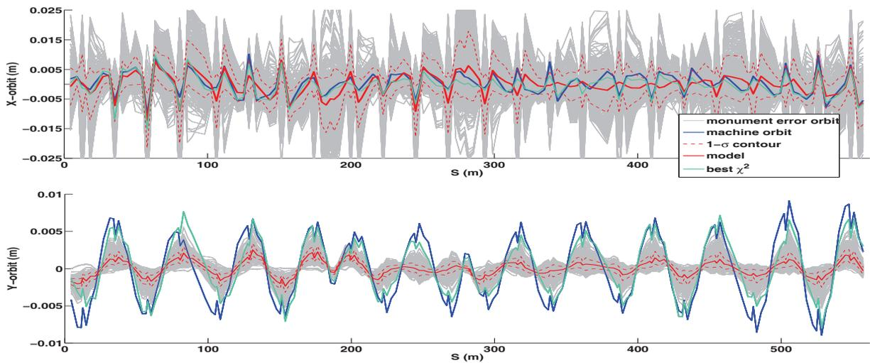
Figure 3: Expected natural orbits from variations in monument positions due to survey instrumental errors for both the planimetric view (top) and the vertical view (bottom).
