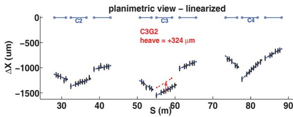
Figure 5: Planimetric view of the zone around cell 3. The sway of +324  $\mu\text{m}$  for girder 2 is shown in red.
