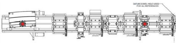
Figure 1: Top view of a standard girder-2. The red dots mark the positions of the monuments used in the survey.
