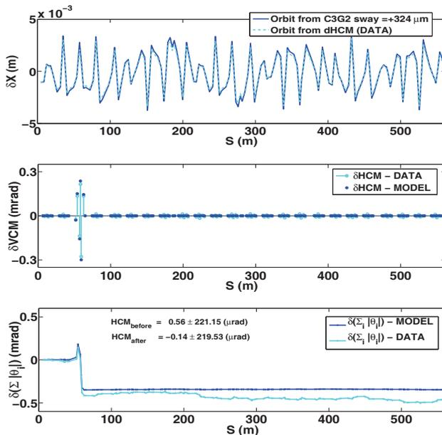
Figure 6: Effects of the horizontal girder displacement as seen in the machine (cyan) and in the model (blue). (Top) Variation in the equilibrium orbit. (Middle) Variation in HCM currents. (Bottom) variation of the integrated CM strength in the storage ring.
