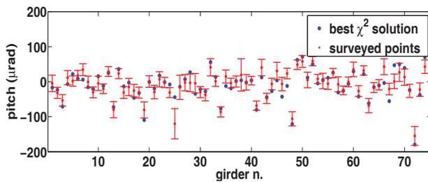
Figure 4: Girder pitch angles. Survey points are shown in red, together with the error bars from instrumental measurements of the monuments. The blue dots show the solution whose vertical orbit better matches the one in the machine.
