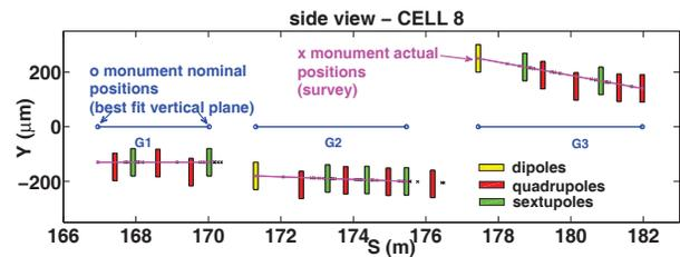
Figure 2: Close-up of the vertical view for cell-8, showing the surveyed magnet displacement for dipoles (yellow), quadrupoles (red) and sextupoles (green). Alignment errors relative to the girder are available for quadrupoles. The magenta lines connect the two survey monuments.
