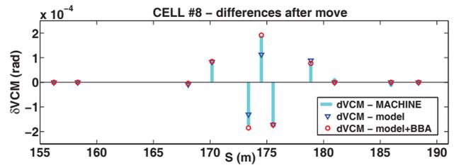
Figure 7: Variation in the vertical correctors of cell 8 after girder 2 heave of +197  $\mu\text{m}$ . (Cyan) data, (blue) orbit corrections with simple girder move model, (red) orbit corrections with the effect of a BBA measurement in the simulation.
