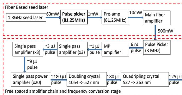
Figure 1: Progression of the photocathode laser system.
