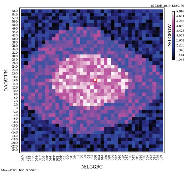
Figure 4: UV intensity map. Horizontal and vertical axis correspond to the green and UV conversion crystal angle respectively.
