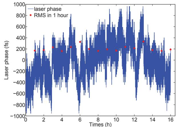
Figure 3: Laser phase measurement over a 16-hour period at steady-state. The blue line is laser phase while the red points represent the standard deviation of the laser phase noise over each hour.
