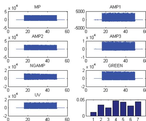
Figure 5: A single capture of 100 bunches on the VME-based digitizer from each of seven photodiodes installed throughout the laser system. The bottom-right corner shows the RMS fluctuation of the amplitude for the pulse train at each stage.
