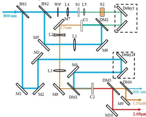
Figure 2: Layout of high-energy 2.05- $\mu\text{m}$  OPA.
