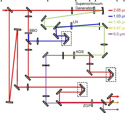
Figure 6: Layout of CEP-stabilized 5-μm OPA.
