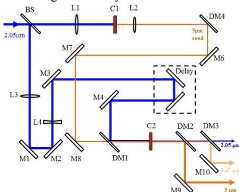
Figure 4: Layout of 5-μm OPA source.
