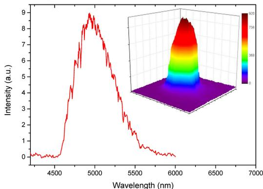
Figure 5: Spectrum and beam profile (inset) of amplified 5-μm pulses.
