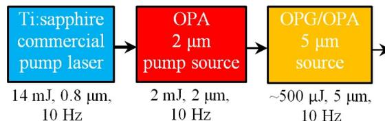
Figure 1: An overview of the technical approach for production of 5  $\mu\text{m}$  pulses.
