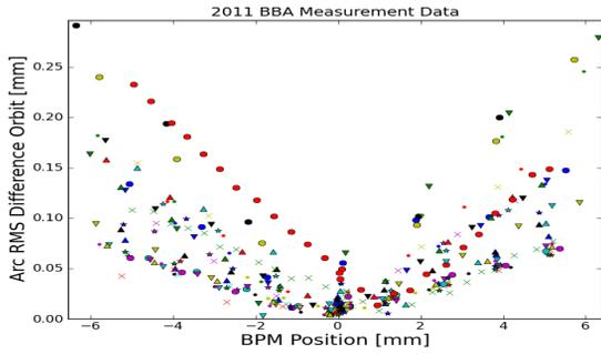
Figure 2: Superimposed BBA measurement data obtained during RHIC 2011 run.
