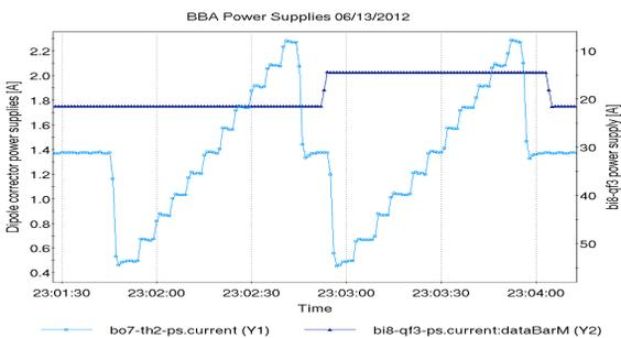
Figure 4: The power supply currents of the same quadrupole and the same dipole corrector as in Figure 3 during BBA measurement with the untypical procedure used during the RHIC 2012 run.
