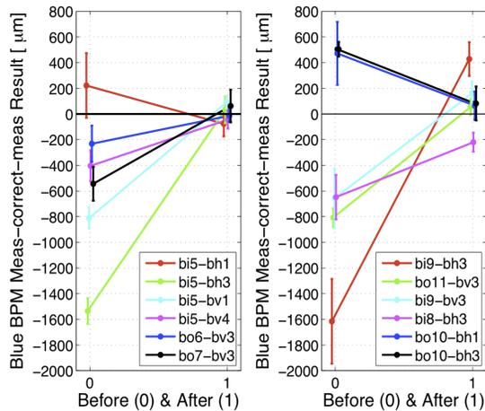
Figure 7: Measurement results before and after the BBA corrections in the Blue ring during RHIC 2012 run.
