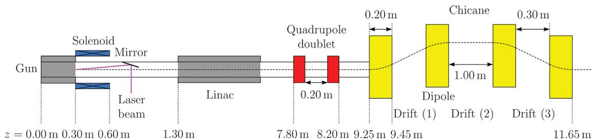
Figure 1: FLUTE baseline layout. In the Buncher scenarios the buncher cavity is placed at 1.3 m and all components are shifted downstream by 2 m or 5 m respectively.
