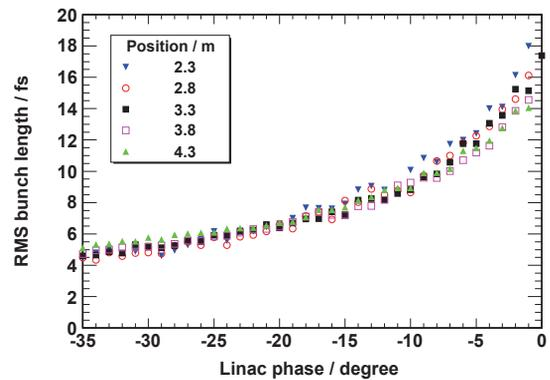
Figure 5: Compressed RMS bunch length vs. the linac phase for different linac positions.
