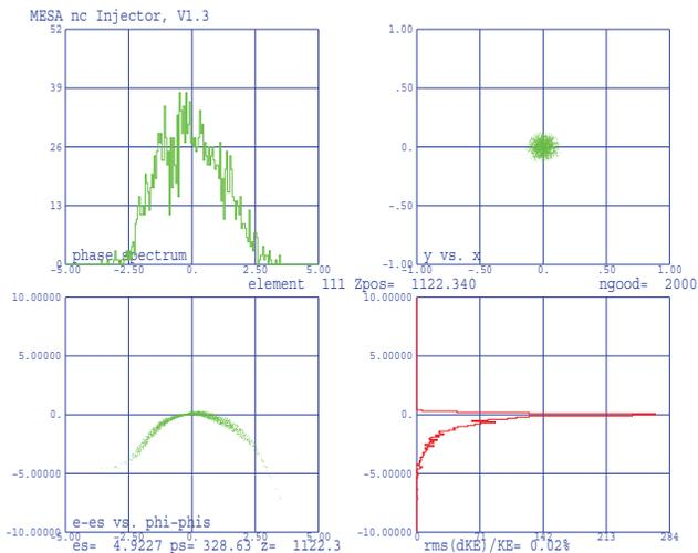
Figure 1: Longitudinal phase space at the end of the nc injector V1.3. The low energy tail of the particle distribution can lead to problems with the main linac sc modules.
