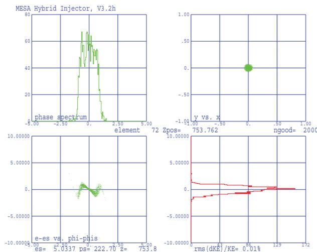
Figure 3: Longitudinal phase space at the end of the hybrid injector V3.2h. This design is the reference design for the hybrid injector.
