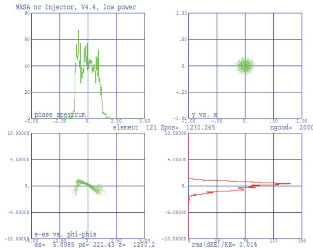
Figure 2: Longitudinal phase space after the last accelerating section of the nc injector V4.4. This design is the reference design for the normal conducting injector.
