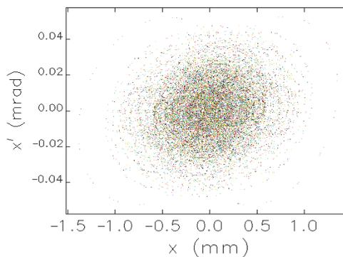
Figure 5: Phase space coordinate of the stored beam monitored after K4. Color indicates to the number of turns.
