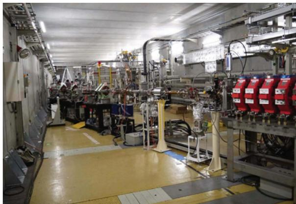
Figure 5: An injector diagnostic beamline.
