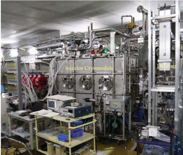
Figure 2: A cryomodule for injector cavities.
