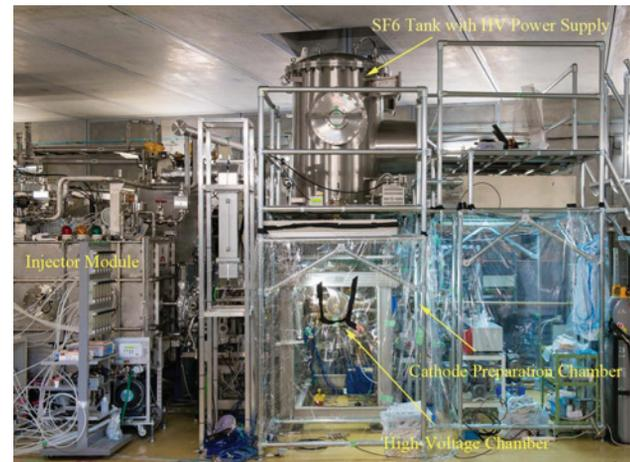
Figure 4: A 500-kV DC photocathode gun.
