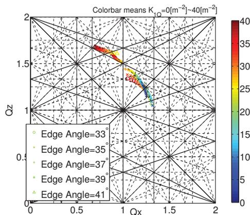
Figure 1: Tune diagram by changing the edge angle of bending magnets and focusing strength of quadrupoles.
