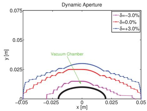
Figure 5: The dynamic aperture for  $\delta = -3.0\%$  (magenta),  $\delta = 0.0\%$  (red),  $\delta = +3.0\%$  (blue). The black half-ellipse is the designed vacuum chamber.
