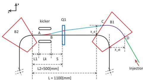
Figure 4: Schematic drawing of the injection process.
