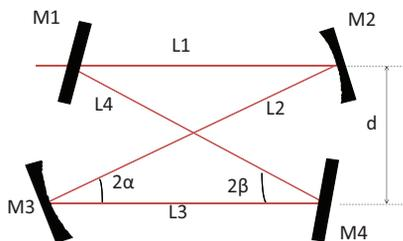
Figure 7: Schematic drawing of the 2D crossed 4-mirror cavity.
