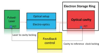
Figure 6: Block diagram of the optical cavity system.
