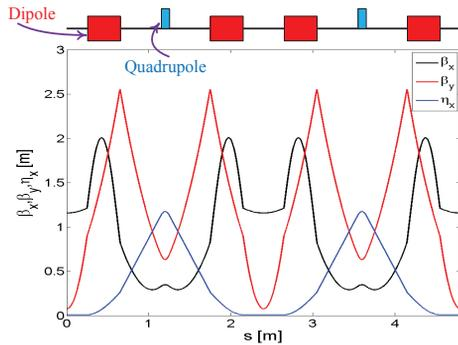
Figure 3: The layout and betatron amplitude function and dispersion function.
