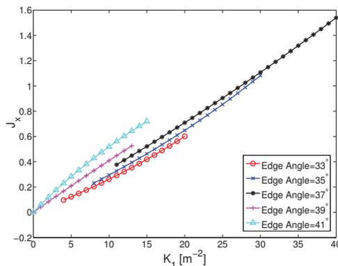
Figure 2: Horizontal damping partition number by changing the strength of quadrupoles at different edge angle.
