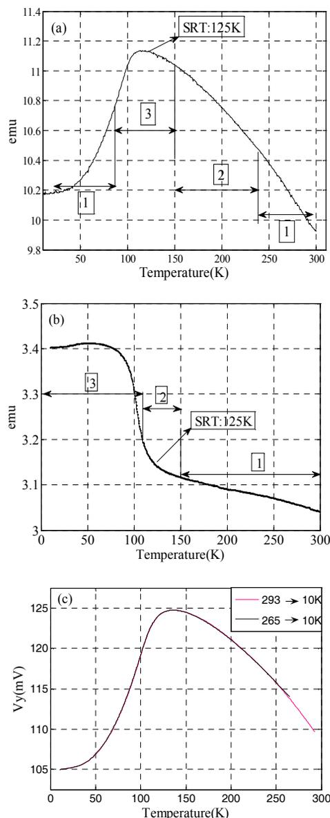
Figure 2: Cryogenic remanence of N50M test results: (a) PPMS: magnet be magnetized and H of PPMS is 0 Gs, magnet size is 2.0mm×2.0mm×2.5mm(orientation is 2.5mm) (b)PPMS: magnet not be magnetized and H of PPMS is 1000 Gs, magnet size is 2.0mm×2.0mm×2.5mm(orientation is 2.5mm) (c) CRMS: magnet be magnetized and H of CRMS is 0 Gs, magnet size is 40.0mm×40.0mm×10.0mm(orientation is 10.0mm) Note: ① emu: total magnetization means  $B_{dr}$  of PM ② Vy: Hall probe voltage means  $B_{dr}$  of PM
