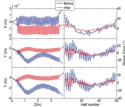
Figure 5: Comparison of on-axis electron trajectories and optical phase errors of EPU104 before (blue) and after (red) shimming. For horizontal polarization shift 0 (top), vertical polarization shift -52mm (middle) and 52mm (bottom) at gap 33 mm.
