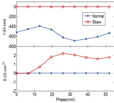
Figure 3: The extrapolated field integral vs. phase at gap 30mm.
