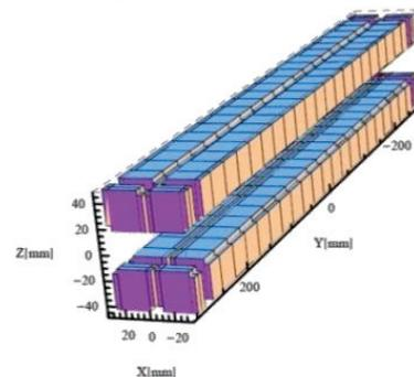
Figure 2: Layout of EPU104 5 periods model.
