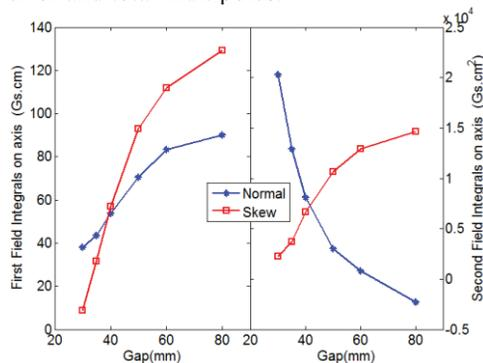
Figure 7: Field integrals of EPU104 as functions of gaps after the correction for both the normal (blue) and skew (red) components.
