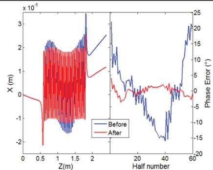
Figure 6: IVU40 Magnetic performances in terms of on-axis electron trajectory (left) and the optical phase error as function of the half period number (right) and before (blue) and after (red) shimming at gap 10 mm.
