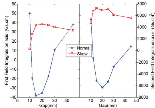
Figure 8: Field integrals of IVU40 as functions of gaps after the correction. For both the normal (blue) and skew (red) components, the effect of the field correction is significant.
