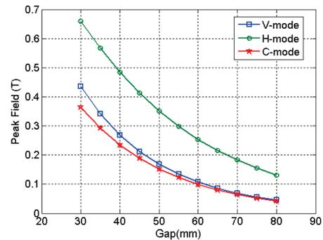
Figure 1: Peak field of three polarizations vs. gaps.
