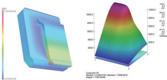
Figure 4: Layout of 1/4 period model and magnetic flux density distribution on the magnetic mid plane.
