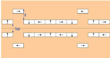
Figure 3: The quasi-periodic design of LEID is performed by vertically translating a few H-magnets by a value  $d$ .
