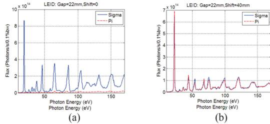
Figure 5: The simulated flux spectrum of LEID in the window  $0.36 \times 0.36\text{mrad}^2$  at min. gap in (a) H.P. Mode and (b) C.P. Mode.
