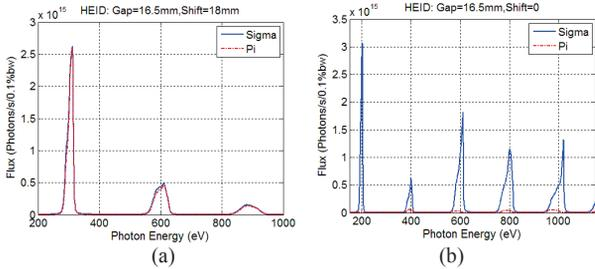
Figure 7: The simulated flux spectrum of HEID in the window  $0.14 \times 0.22 \text{mrad}^2$  at gap 16.5mm in (a) H.P. Mode and (b) C.P. Mode.
