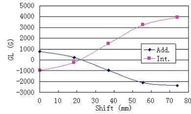
Figure 8: The intrinsic/additional quadrupoles of LEID vs. magnet array shift.
