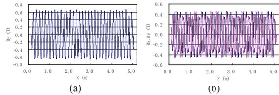
Figure 4: The quasi-periodic magnetic fields on axis of LEID at minimum gap of 22mm in (a) H.P. Mode and (b) C.P. Mode.
