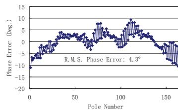
Figure 6: The phase error distribution of HEID at gap 16.5mm in H.P. Mode.
