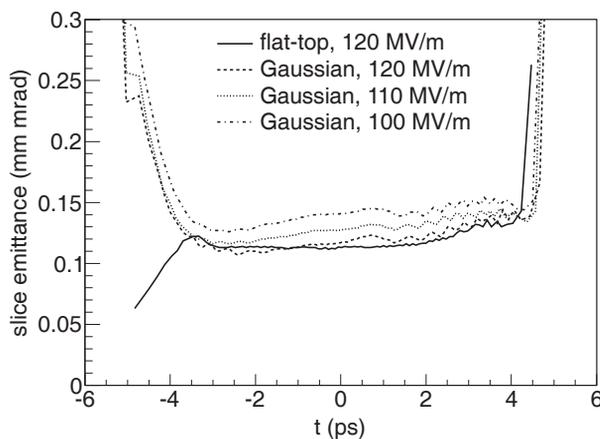
Figure 2: Slice emittance at the injector end for operation conditions using different longitudinal drive-laser profile and RF field at the cathode.
