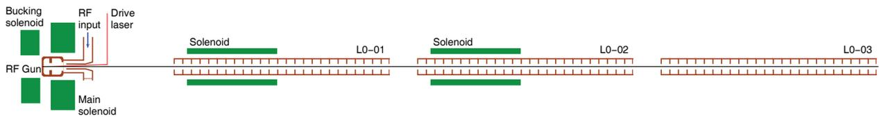
Figure 1: Layout of the low emittance injector consisting of an RF photocathode gun, focusing solenoids, and three accelerating sections.
