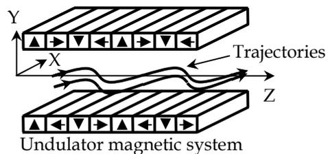
Figure 1: Sketch of a permanent magnet undulator.
