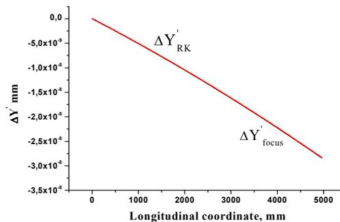
Figure 5. Focusing vs. numerically simulated components of vertical velocity.
