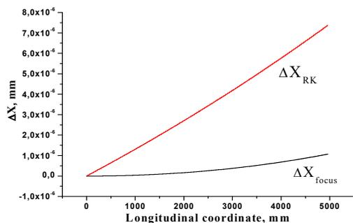
Figure 2. Focusing vs. numerically simulated components of horizontal coordinate.
