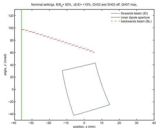
Figure 5: ID beamlines: phase space boundaries at the entrance to the bending in the worst combination of errors.
