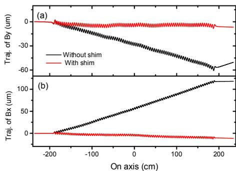
Figure 2: Trajectory of the electron beam on axis at a circular polarization mode. (a) Trajectory of  $B_y$ . (b) Trajectory of  $B_x$ .
