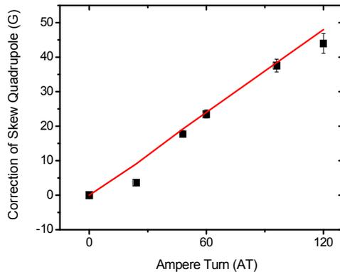
Figure 6: Correction of the skew quadrupole term using long coils. Squares mark the experimental data; the solid line is from the simulation.
