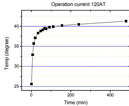
Figure 7: Temperature variation of long coils operating at 120 AT.
