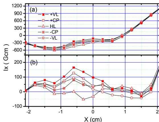
Figure 5: First integral of horizontal field ( $I_x$ ) along the longitudinal direction (a) without, and (b) with, the magic finger correction.
