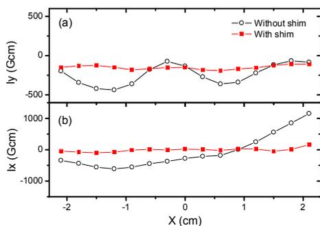
Figure 4: Distribution of the first integral of horizontal ( $I_x$ ) and vertical field ( $I_y$ ) for the circular polarization mode.
