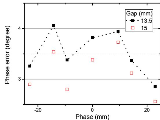
Figure 1: r.m.s. phase error as a function of gap and phase.
