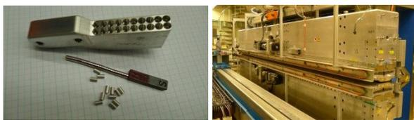
Figure 3: Two methods to correct multipole error. (a) A magic finger structure, magnet chips and aluminium spacers. (b) A long coil loop.
