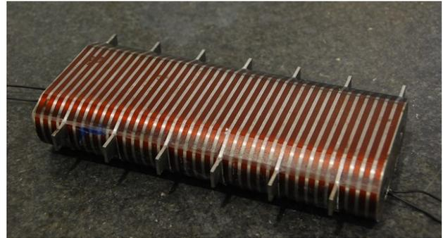
Figure 1: Fully wound and potted magnet array awaiting magnet tests.
