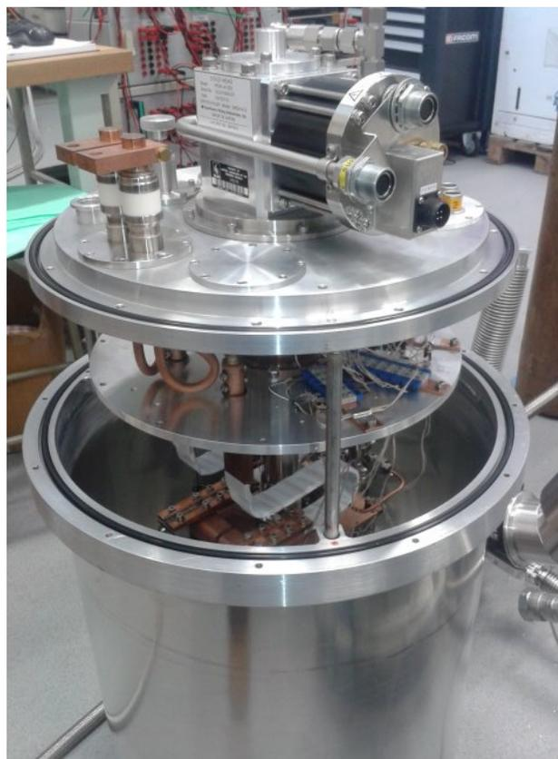
Figure 3: Cryogenic turret assembly prior to testing.
