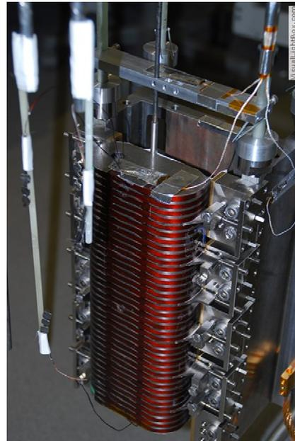
Figure 2: Magnet array mounted vertically for 4.2 K magnet tests.
