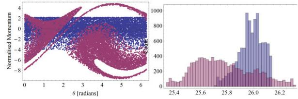
Figure 3: Normalised Phase space pre- (Blue) and post- (Purple) FEL for one 8 $\mu\text{m}$  wavelength bunchlet (left) and the resulting change in bunch energy spread for the entire bunch (right).
