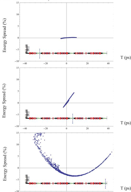
Figure 8: Longitudinal phase space at the exit of the 2<sup>nd</sup> linac cavity for each of the 3-passes at 60 pC.
