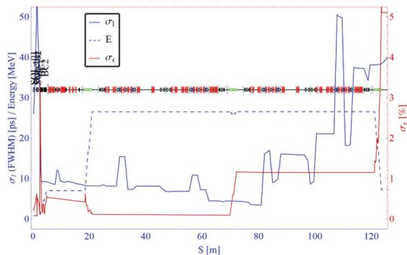
Figure 6: Longitudinal beam properties for 2-loop ALICE ERL at 60 pC.
