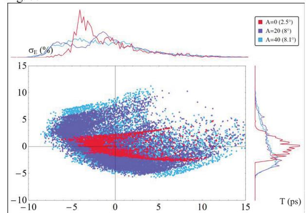
Figure 5: Bunch length (ps) vs. relative energy spread (%) distributions, after the return linac deceleration, for 3 different FEL powers.
