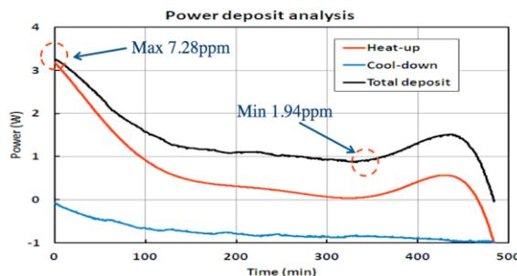
Figure 5: Analysis of beam power deposited into the beam block through 2 mm beam tube test based on data in Fig. 4.
