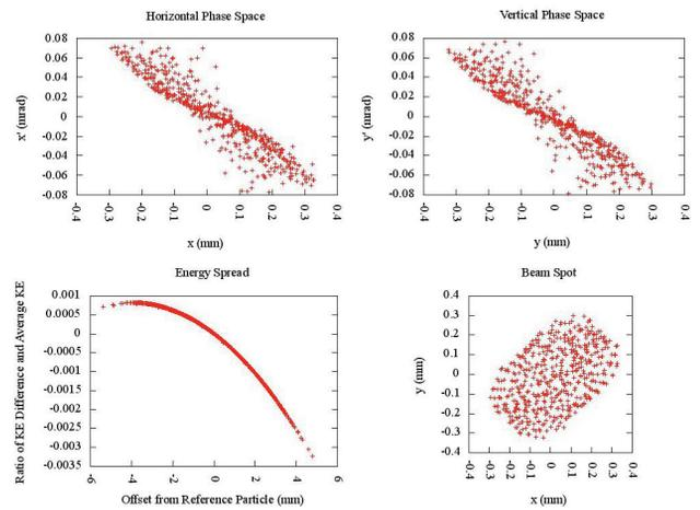
Figure 4: Beam distribution at linac exit, E=25 MeV.
