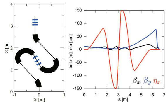
Figure 5: Magnetic bunch compressor footprint (left) and optics (right). The compressor fits within a  $2.0\text{m} \times 3.5\text{m}$  space, and provides large dispersion for sextupole chromatic and  $T_{566}$  control.
