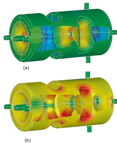
Figure 2: (a) Surface electric field and (b) surface magnetic field for the 500 MHz  $\beta = 1$  double spoke cavity.
