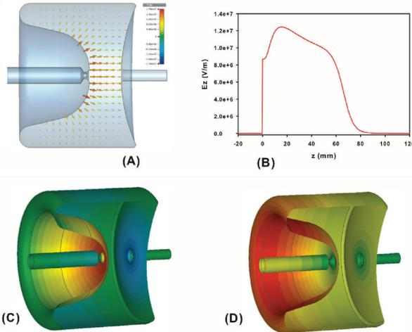
Figure 1: Preliminary design of a 500 MHz quarter wave electron gun. (A) Longitudinal cross section and electric field within the cavity at 1 J (B) Accelerating electric field profile along beam axis; (C) Surface electric field; (D) Surface magnetic field.
