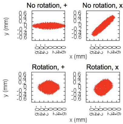
Figure 3: Spoke cavity orientation effects on beam distribution at end of linac. “+” and “x” are spoke orientations. “Rotation” alternates spoke orientation by  $90^\circ$  between successive cavities, while “No rotation” does not. Nearly round uncoupled beam is provided by the “Rotation +” configuration.
