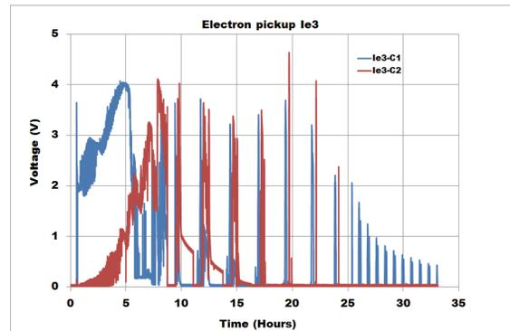
Figure 8: Electron pickup current measurement (converted to voltage:  $1\mu A \rightarrow 1V$ ) on cold parts during RF conditioning.
