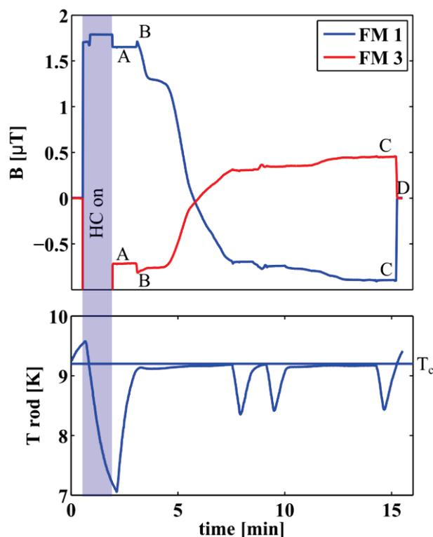
Figure 2: Behavior of trapped flux and temperature when a HC field of  $33\mu T$  is applied and trapped: Initially trapped flux (A), reduced trapped flux (C) and level of flux ambient in  $HoBiCaT \approx 3\mu T$  (D). This value has been subtracted from all data points.
