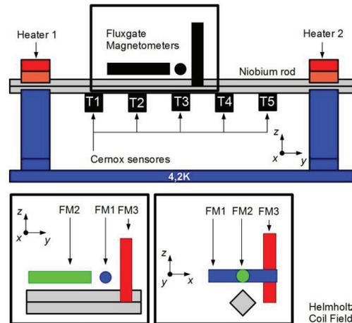
Figure 1: Experimental setup and position of instruments: Longitudinal view (left) and cross section (right) of FM1 (black), FM2 (green) and FM3 (red).
