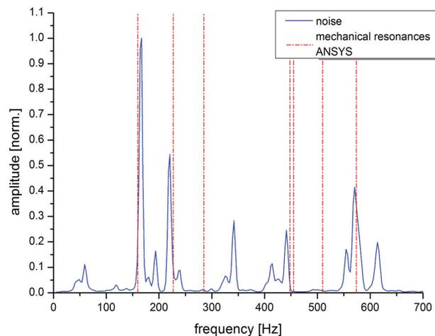
Figure 4: Comparison between sweeping method and white noise technique (top) and between measurements and ANSYS simulation results (bottom).
