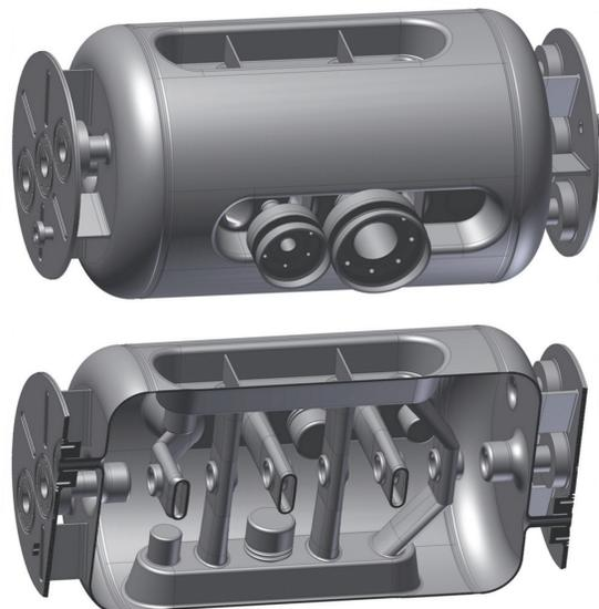
Figure 1: Layout of the sc 325 MHz CH-cavity [1].
