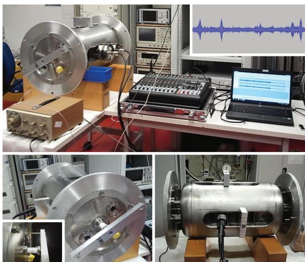
Figure 3: Test setup for microphonics measurements in the environment of the cryo-lab at the IAP, University of Frankfurt.
