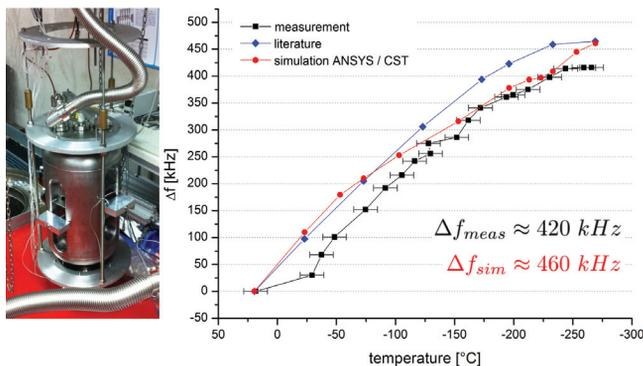
Figure 6: Prepared cavity before cool down (left) and comparison between simulated and measured frequency shift due to cool down (right).
