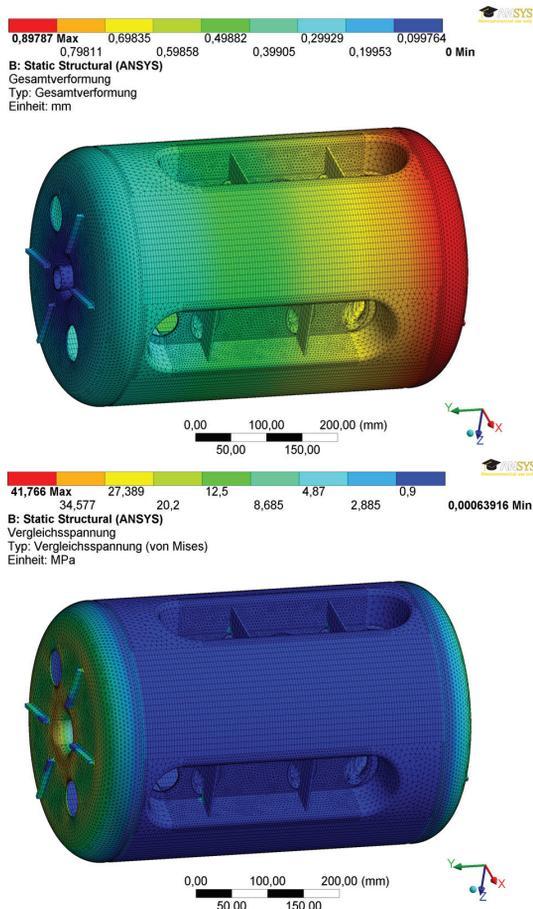
Figure 5: Displacement of the cavity walls caused by cool down (top) and appearing von-Mises stress (bottom).
