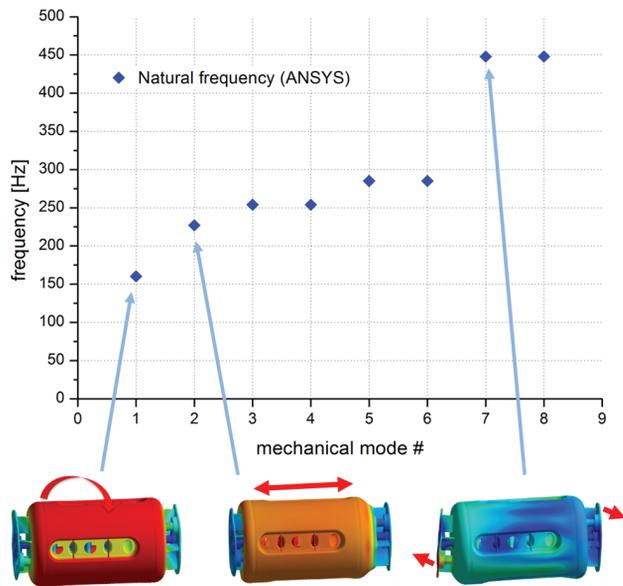
Figure 2: Simulated natural frequencies and three of the corresponding oscillation modes of the sc 325 MHz CH-cavity.
