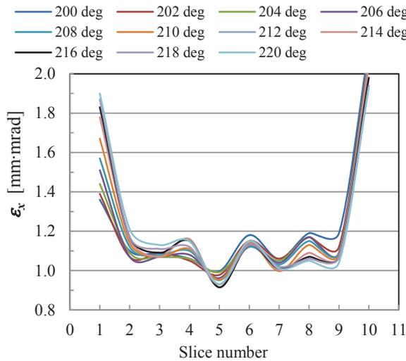
Figure 6: (Color) Slice emittance  $\epsilon_x$  for different irradiation phase. Result for  $\epsilon_y$  was very similar.
