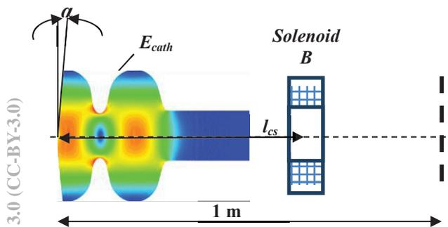
Figure 1: (Color) Layout of the SRF injector with the Tesla-type 1.6-cell cavity and solenoid.
