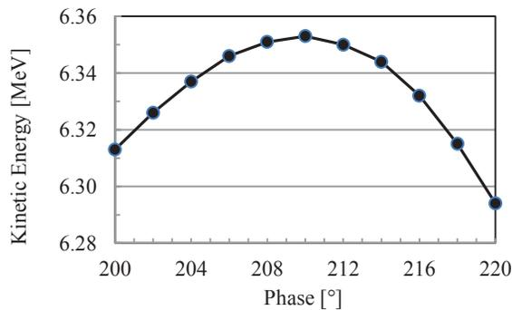
Figure 7: (Color) Kinetic energy vs. phase.
