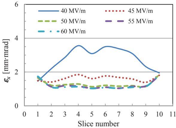
Figure 3: (Color) Slice emittance  $\epsilon_x$  vs.  $E_{cath}$ .
