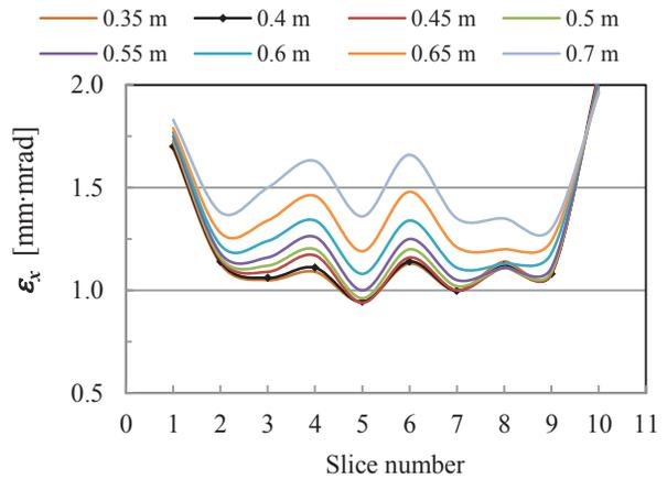
Figure 8: (Color) Slice emittance  $\epsilon_x$  for different position of solenoid.
