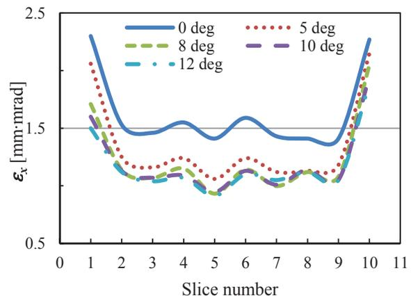
Figure 2: (Color) Slice emittance  $\epsilon_x$  for different  $\alpha$ .
