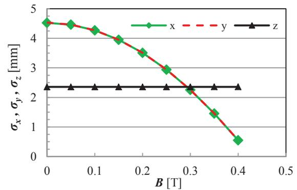
Figure 5: (Color) Bunch size for different  $B$  values. Note the overlapping of  $\sigma_x$  and  $\sigma_y$ .
