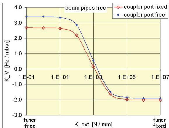
Figure 7: cHWR under external pressure with different coupler port constraints and tuner stiffness variation (beam pipes free).
