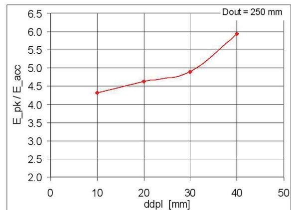
Figure 5: cHWR-250 surface peak electrical field.
