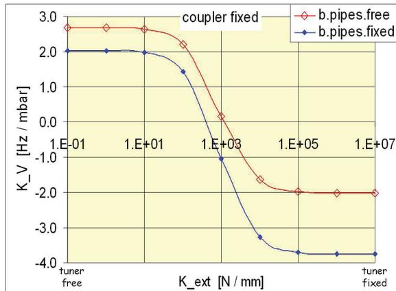
Figure 6: cHWR under external pressure with different beam port constraints and tuner stiffness variation (coupler port fixed).
