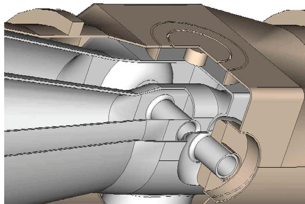
Figure 9: cHWR simulation model with bellow slot.
