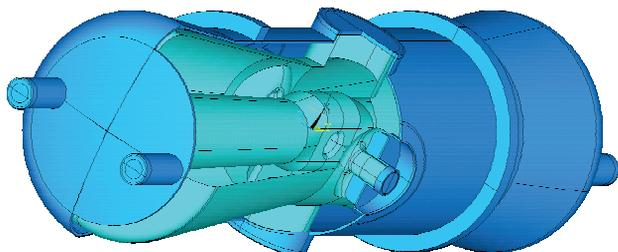
Figure 1: Simulation model of cylindrical cHWR with helium vessel.
