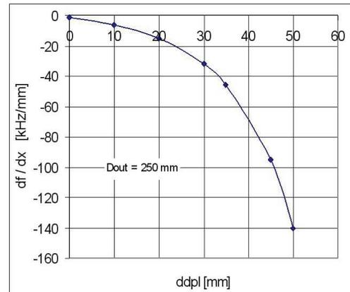
Figure 4: cHWR-250 with helium vessel tuning sensitivity.
