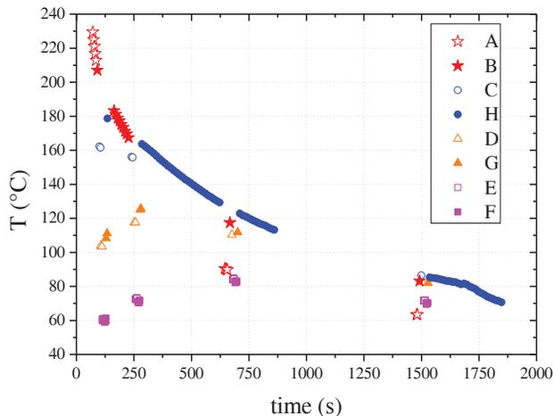
Figure 3: Temperature at different locations of the two-cell cavity. For dot positions see Fig. 2.
