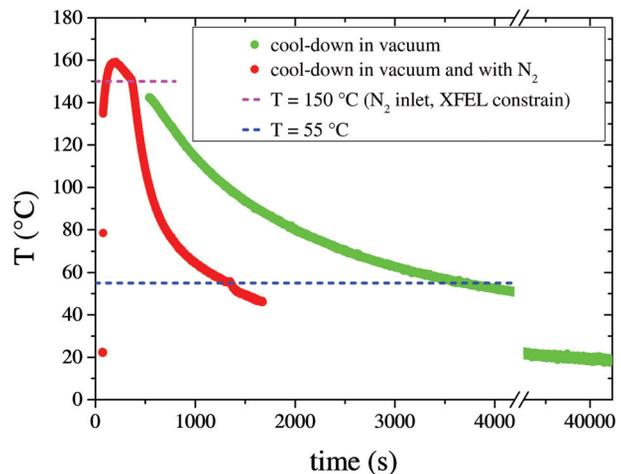
Figure 4: ECU cooling without and with N<sub>2</sub>. Magenta line represents the XFEL prescription for starting venting the EBW machine with N<sub>2</sub>.
