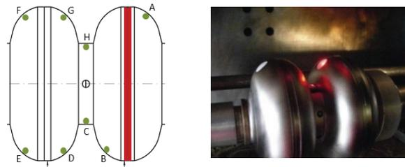
Figure 2: Positions of the “emissive dots” and photo during measurement: red laser beams are used for alignment.
