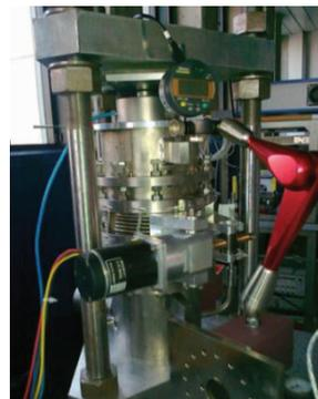
Figure 9: Setup for testing 3.9 GHz coaxial tuner units.
