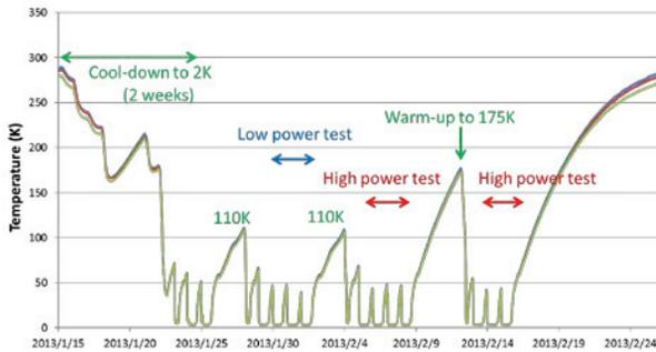
Figure 3: Cavity temperature during cool-down tests.
