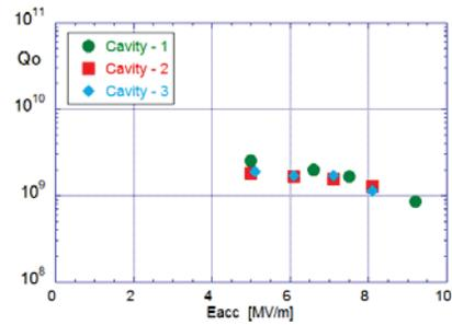
Figure 8: Measured  $Q_o$  values of three cavities in a CW operation at 2 K.
