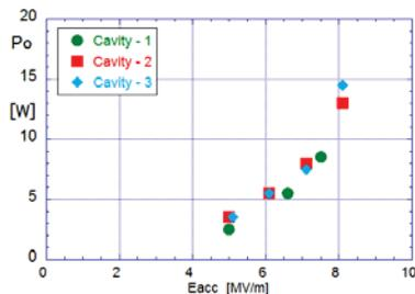
Figure 7: Cavity dynamic heat load ( $P_o$ ) measured by a evaporated He-gas flow at 2 K.
