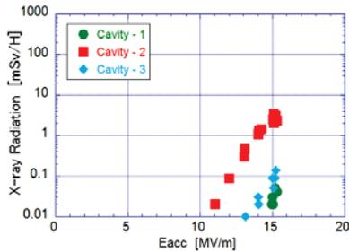
Figure 6: X-rays radiation observed in a pulsed operation with 50 ms and 2 Hz (duty 10 %) in a single cavity operation of three cavities.
