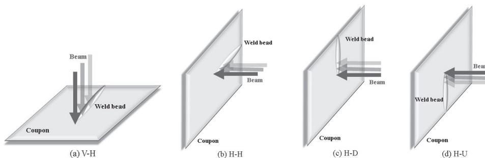
Figure 1: Schematic layouts of combinations of a generator position and a welding direction. (a) V-H: the vertical generator position and the horizontal welding direction, (b) H-H: the horizontal generator position and the horizontal welding direction. (c) H-D: the horizontal generator position and the downward welding direction, and (d) H-U: the horizontal generator position and the upward welding direction.
