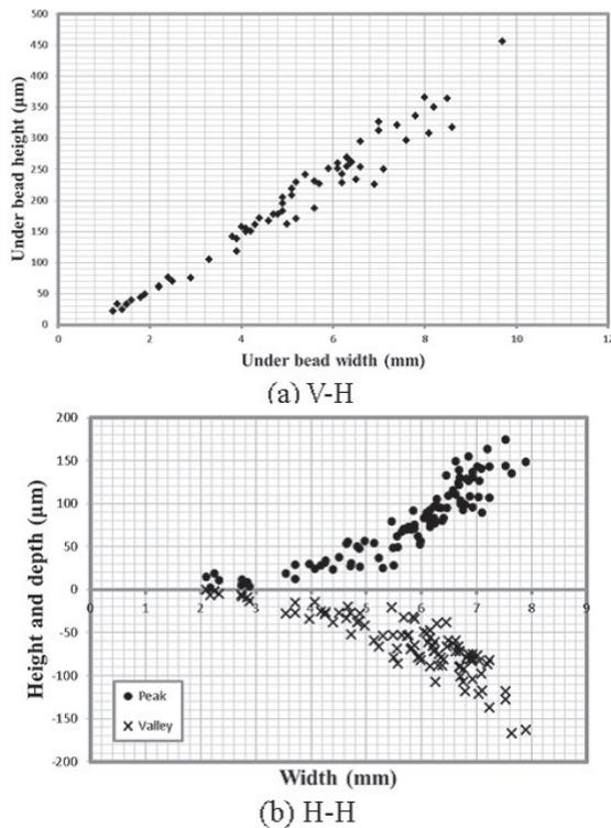
Figure 3: (a) A relation between a peak height and an underbead width for the combination V-H. (b) A relation among a peak height, a valley depth and an underbead width for the combination H-H. The EBW parameters are varied as shown in Table 1 except for the generator position and the welding direction.
