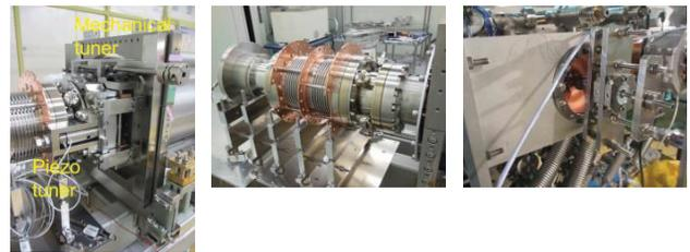
Figure 7: (left) Frequency tuner, (center) HOM absorber and (right) input coupler.
