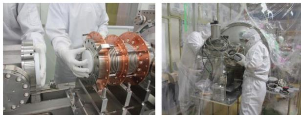
Figure 3: Connection of HOM absorber (left) and gate valve (right).
