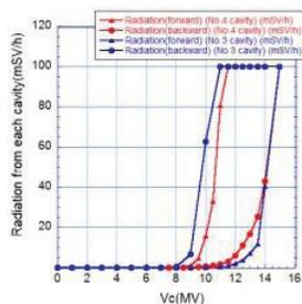
Figure 10: Measured accelerating voltage ( $V_c$ ) and radiation doses for both cavities.
