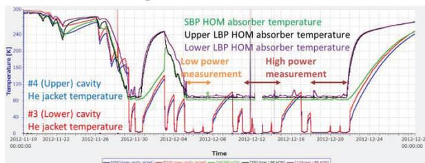
Figure 6: Cooling history of the cryomodule.
