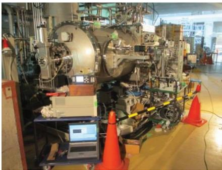
Figure 5: Main linac cryomodule placed inside radiation shield of cERL.
