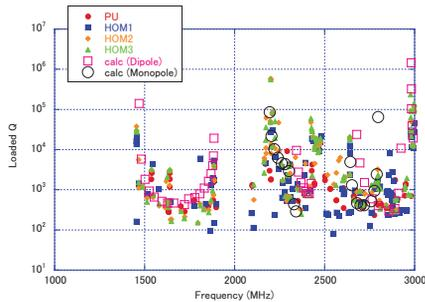
Figure 9: Measured HOM characteristics for #3 cavity, compared with calculated ones. PU means fundamental pickup antenna and HOM1, HOM2 and HOM3 mean HOM probes.
