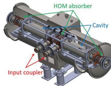
Figure 2: Schematic view of ERL main linac cryomodule.
