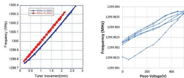
Figure 8: Performances of the mechanical tuners (left) and piezo tuners (right).
