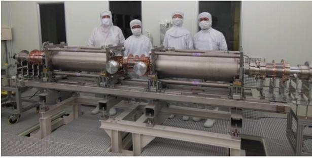
Figure 4: After completion of cavity string assembly.
