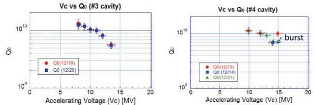
Figure 11: Measured  $Q_0$  values for #3 cavity (left) and #4 cavity (right).
