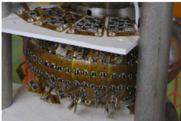
Figure 5: Installed XT-map leaves on a cell. X-sensors are mounted on outer side. Multiplexers, peripherals and connections are on the base of the leaves.
