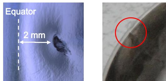
Figure 3: Quench defect in cell#9 (left), grain boundary step of the half cell after pressing and trimming (right).
