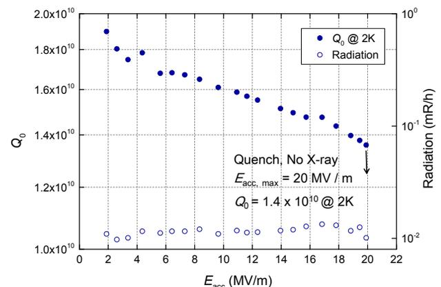
Figure 2: Test result of the IHEP-02 LL LG cavity.
