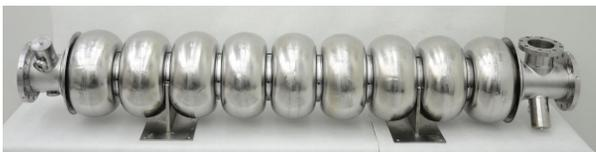
Figure 1: IHEP-01 low-loss large grain 9-cell cavity.
