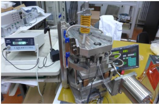
Figure 8: Tuner in the room temperature test stand.
