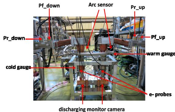
Figure 5: High power test stand.
