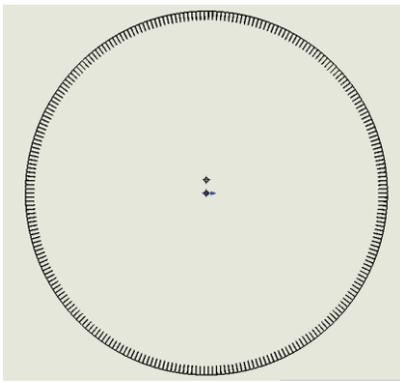
Figure 4: The top view of the beryllium bronze contact plate with about 270 slots in the equator area for sufficient electrical contact.
