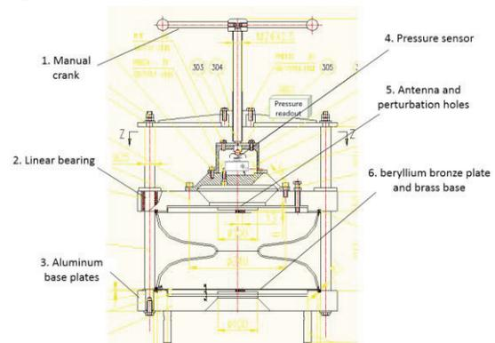
Figure 3: Mechanical design drawing of the setup.
