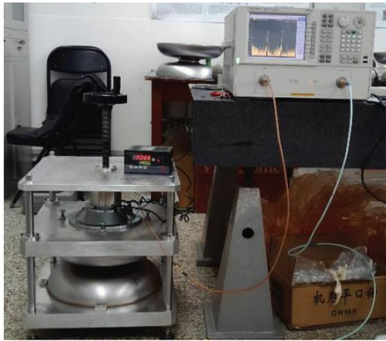
Figure 8: The photo of frequency measurement setup.
