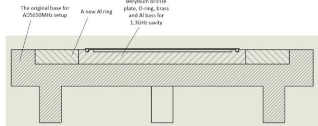
Figure 6: Schematic of the setup modification for 1.3GHz cavities.
