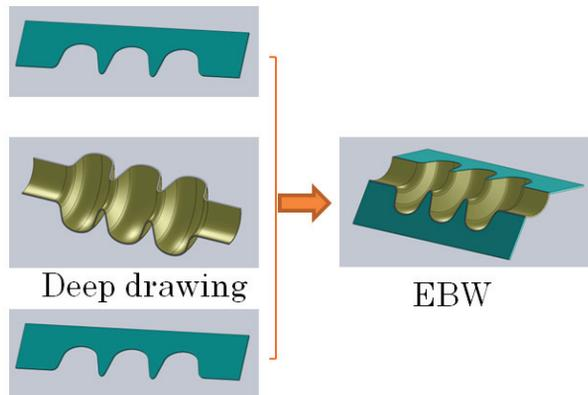
Figure 5: The mechanical structure of the slotted cavity (up) and the fabrication method (down).
