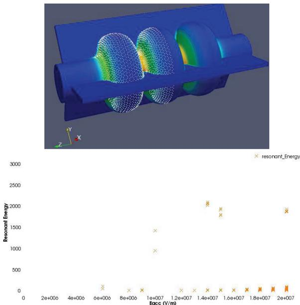
Figure 3: The initial emitting points in the cavity (up). The impact energy versus  $E_{acc}$  of the 1.3GHz slotted cavity (down).
