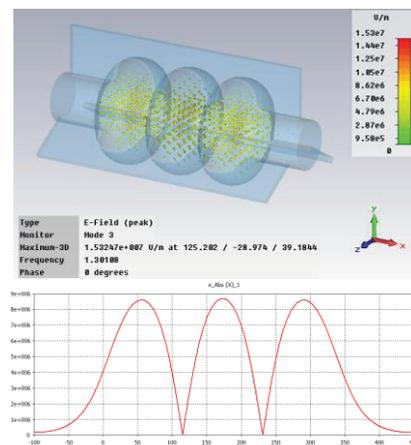
Figure 1: Electric field of  $\pi$  mode in the cavity (up). The field flatness of  $\pi$  mode (down).
