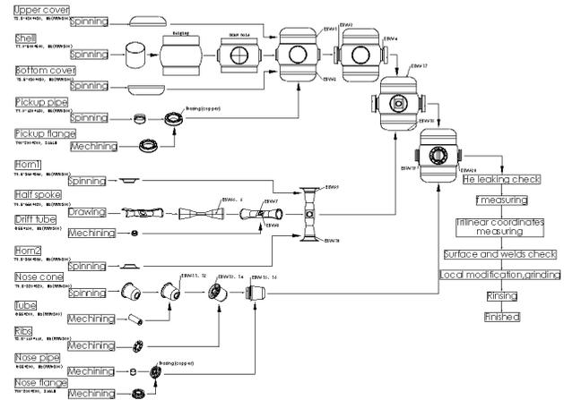
Figure 9: The fabrication sequence of the cavity.
