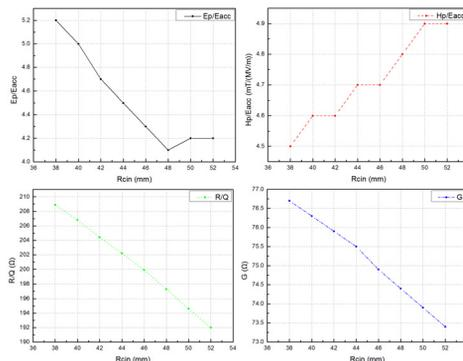
Figure 2: The sweep results of inner radius of nose cone.
