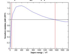
Figure 5: SEY curve for Niobium of 300°C bake out.
