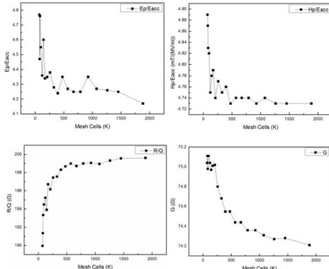
Figure 4: RF parameters' convergence of mesh cells.
