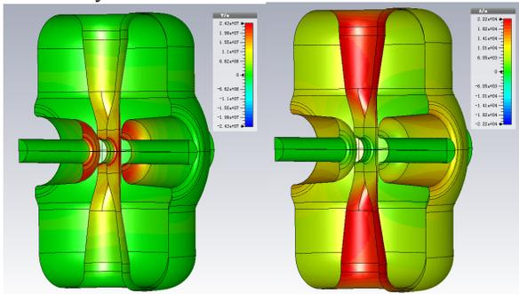
Figure 3: Electric field distribution (left) and magnetic field distribution (right) of the cavity.
