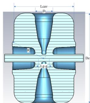
Figure 1: The cross section of the cavity with the main geometric parameters:  $L_{cav}=274$  mm;  $D= 80$  mm;  $D_{cav}=405.6$  mm;  $R=160$  mm;  $L_{g-g}=\beta \lambda/2=55$  mm.
