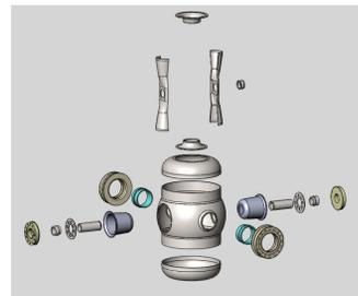
Figure 8: The exploded view of the cavity.
