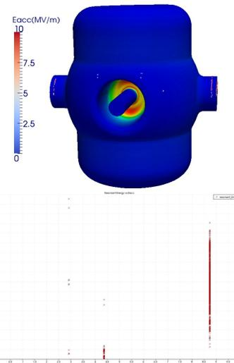
Figure 6: Multipacting location (upper) and multipacting resonant energy VS.  $E_{acc}$  (bottom) results from Track3P.
