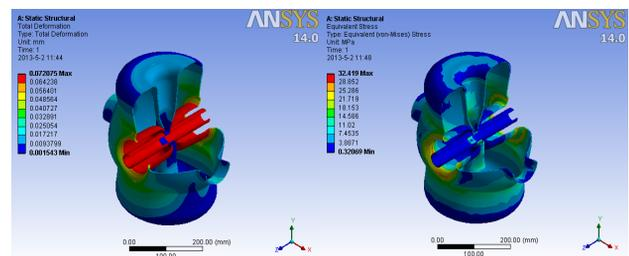
Figure 7: Simulation of deformation (left) and stress (right) for the cavity at 2 bar, and all the port are free.
