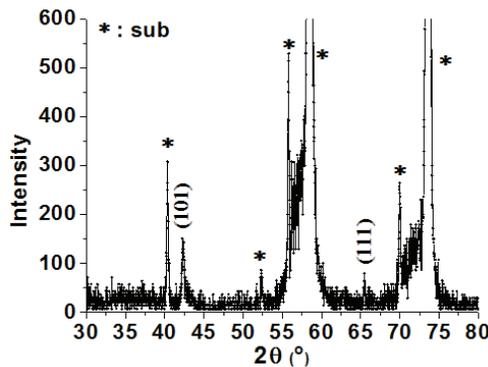
Figure 2: X-ray diffraction patterns of  $10 \times 10 \text{ mm}^2$   $\text{MgB}_2$  film.
