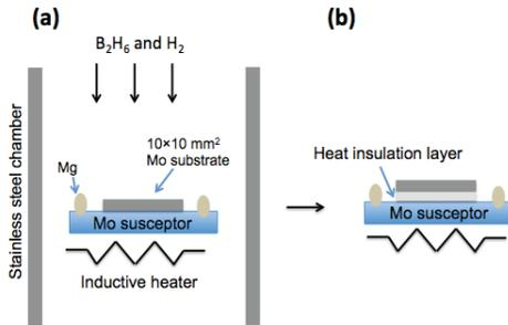
Figure 1: Schematics of (a) HPCVD equipment and (b) heat insulation layer.
