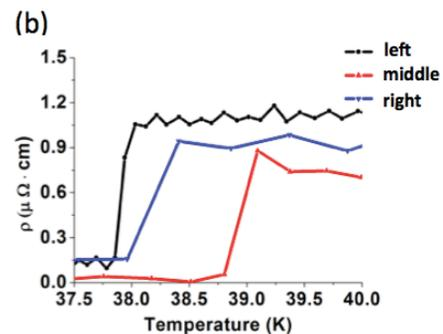
Figure 4: (a) Resistivity versus temperature curve for the middle one of three pieces, (b) Resistivity versus temperature curves nearby the transition region of three pieces.
