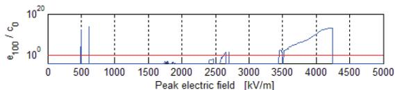
Figure 5: The plot of enhanced counter function. Multipacting occurs at peak surface electric field 494-498, 612-614, 2568-2650, 2700-2704, 3426-3500 and 3520-4250 kV/m.
