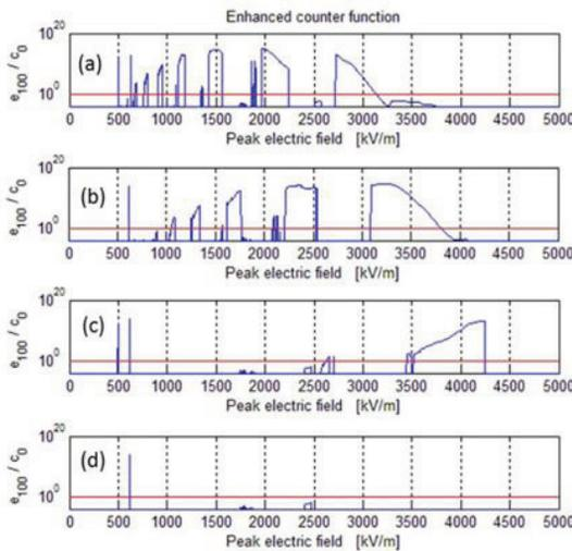
Figure 7: Enhanced counter function plot for different radius of the corner in the open end of the cavity. (a) R=30 mm. (b) R=20 mm. (c) R=5 mm. (d) R=2 mm.
