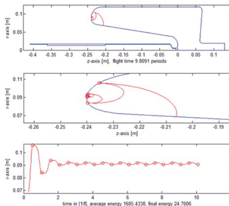
Figure 4: The electron trajectory at 17.5 MV/m. The top figure represents the trajectory of the electron in  $(r, z)$  coordinates, the middle one is an expanded plot of a part of the top one, and the bottom plot illustrates the electron's trajectory in the  $(r, t)$  coordinates where  $t$  is the time in rf periods. The circles indicate the impacts on the walls of the cavity.
