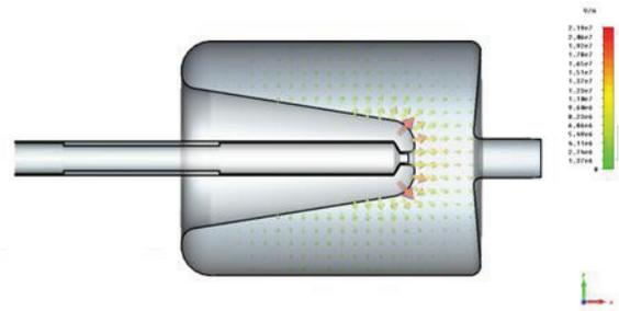
Figure 1: Longitudinal cross section and electric field within the cavity.
