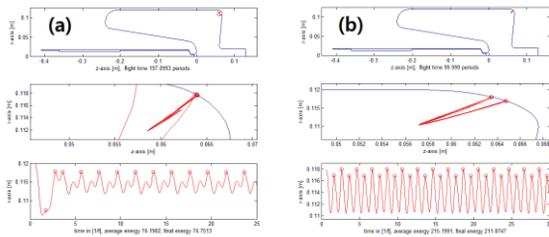
Figure 6: Two types of MP trajectories from Multipac results. (a) The second-order single-point MP at peak surface electric fields 2700kV/m. (b) The first-order two-point MP at peak surface electric fields 4000kV/m.
