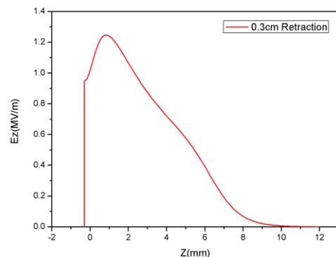
Figure 2: Accelerating electric field profile along beam axis.
