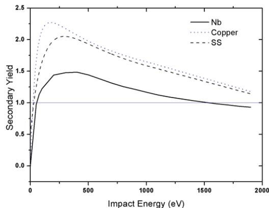
Figure 3: Secondary electron yield for niobium, copper and stainless steel as a function of the electron impact energy in eV.
