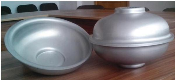
Figure 5: First half-cells made of aluminium by hydraulic deep drawing in Minsk.
