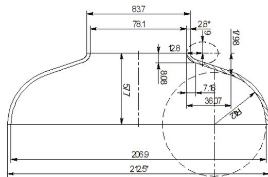
Figure 1: Shape of half-cell.
