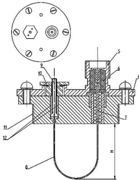
Figure 2: Coupling device.
