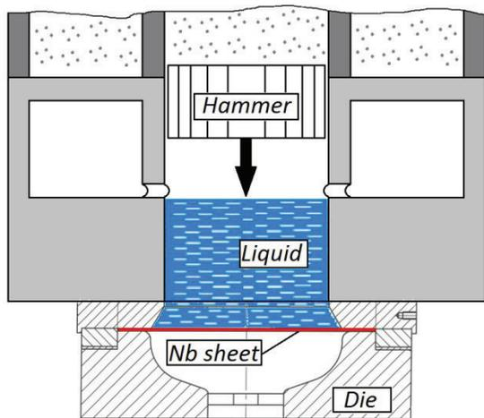
Figure 4: Scheme of hydraulic deep drawing.
