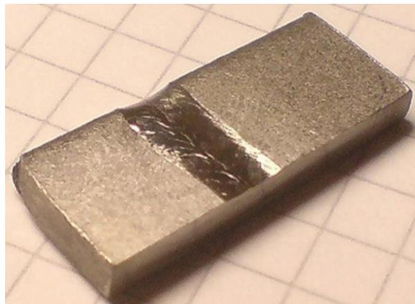
Figure 6: Sample of EBW of niobium in Minsk.
